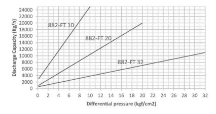
Note: Capacities shown are based on discharge at saturation temperature. In 882FT when discharging sub-cooled condensate, the air vent provides extra capacity. Under start up conditions, the air venting will be open, and will provide additional condensate capacity to outlet.
