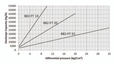
Note: Capacities shown are based on discharge at saturation temperature. In 882FT when discharging sub-cooled condensate, the air vent provides extra capacity. Under start up conditions, the air venting will be open, and will provide additional condensate capacity to outlet.
