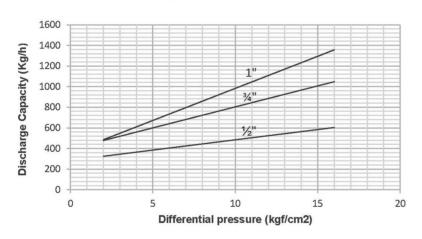
Note: Traps should be selected for the most appropriate working pressure differential and not on the basis of load.
